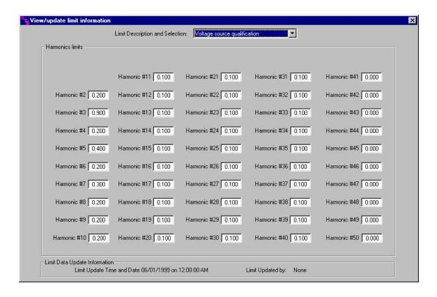
During current harmonics testing, the voltage distortion of the AC Source or Line voltage is constantly monitored by the PCTS system. The EN 61000-2-3 voltage distortion test limits are displayed in this screen and can be modified if and when a new standard is issued that applies different limits.
